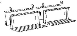
(1.) SCREW BRACES TO TOP AS SHOWN (LOOSE, DO NOT TIGHTEN)
