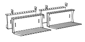
(1.) SCREW BRACES TO TOP AS SHOWN (LOOSE, DO NOT TIGHTEN)
