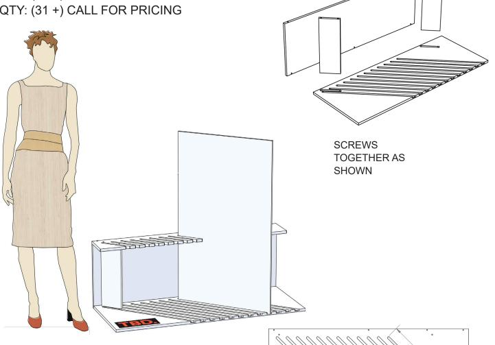
HOLDS (12) SAMPLES, SIZES 24" X 48" HOLDS SAMPLES UP TO 1/2" THICK. WHITE WITH WHITE PAINTED EDGES LEFT OR RIGHT VERSIONS AVAILABLE WE CAN MAKE OTHER SIZE SLOTS WEIGHT" 30LBS
