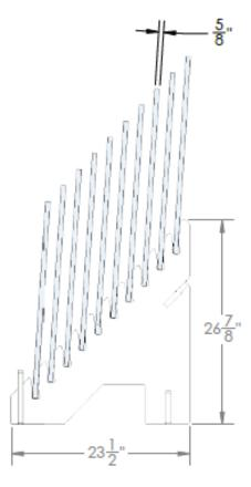
HOLDS 10 SAMPLES MINIMUM WIDTH 14"WIDTH, WHITE WITH WHITE PAINTED EDGES MAXIMUM TILE THICKNESS IS 5/8" WE CAN MAKE OTHER SIZE SLOTS FOOTPRINT: 13" WIDE X 23-1/2" DEEP X 26-7/8" TALL
