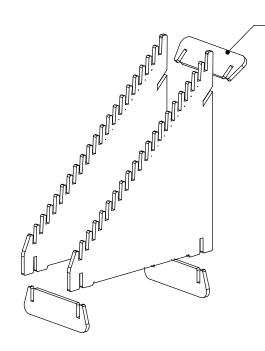
SIMPLE "SLIP-TOGETHER" ASSEMBLY (NO TOOLS REQUIRED)
