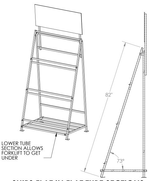
SHIPS FLAT IN FLAT TUBE SECTIONS THEN ASSEMBLE ON-SITE WITH BOLTS
